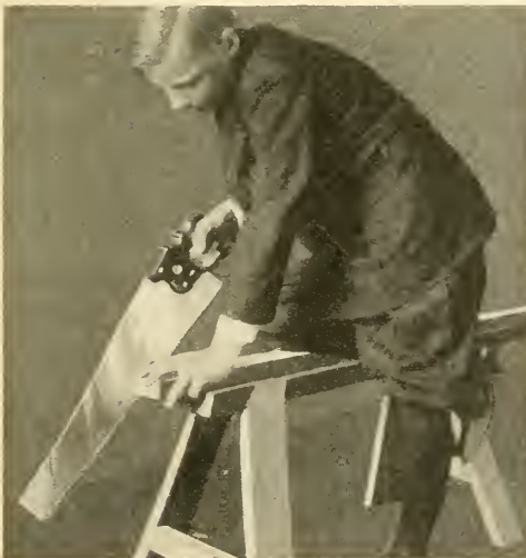
Fig. 15. Ripsawing on a Saw Horse.
